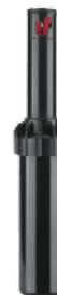
PGJ-04 Overall height: 18 cm Pop-up height: 10 cm Exposed diameter: 3 cm Inlet size: ½"
