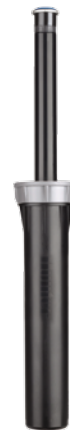
PROS-06-PRS40-CV Retracted height: 22.5 cm Pop-up height: 15 cm Exposed diameter: 5.7 cm Inlet size: 1/2"
